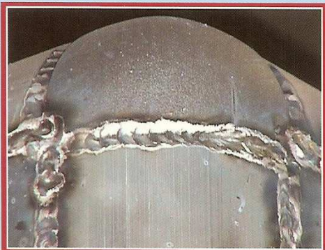
All seams continuously welded
