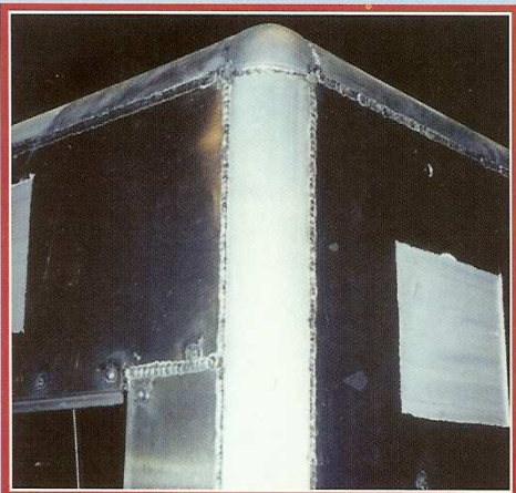
All seams continuously welded
