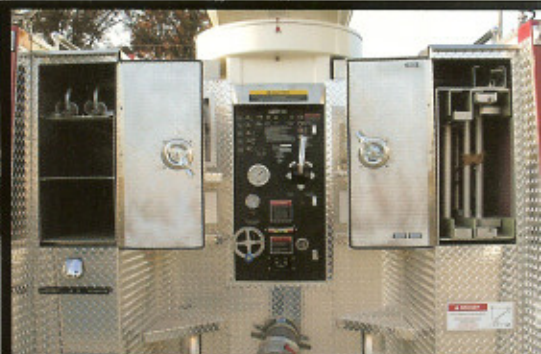
Equipment storage and full aerial controls at rear
