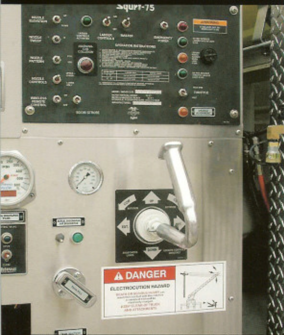
Integrated pump panel controls for easy operation
