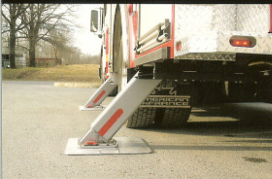
Minimal outrigger spread
