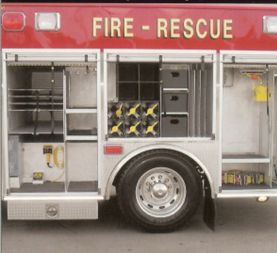
Wheel well compartment, pvc toolboxes, and bottle storage
