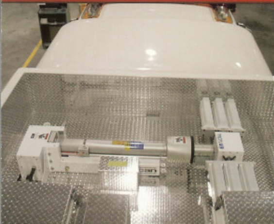
Recessed light tower mounting
